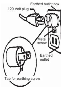
An adaptor must be installed as shown here if only two prong outlets are available. The outlet box must be earthed and the earthing tab (or wire) must be installed under the head of the centre screw at the outlet cover. 120 Volt plugs are available at most hardware stores. Earthing adaptors are not approved for use in Canada.
